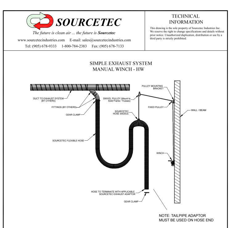
Sourcetec HW Hose and Winch Simple Exhaust System is made up of rope and pulley mechaisms and a wall mounted winch to lift and lower low temp or high temp flexible hose and hose saddle. Sourcetec HW Hose and Winch can be used as a single drop or hung from the main duct for a complete system. Hoses are available in 4" up to 8" Dia and lengths up to 33ft.
