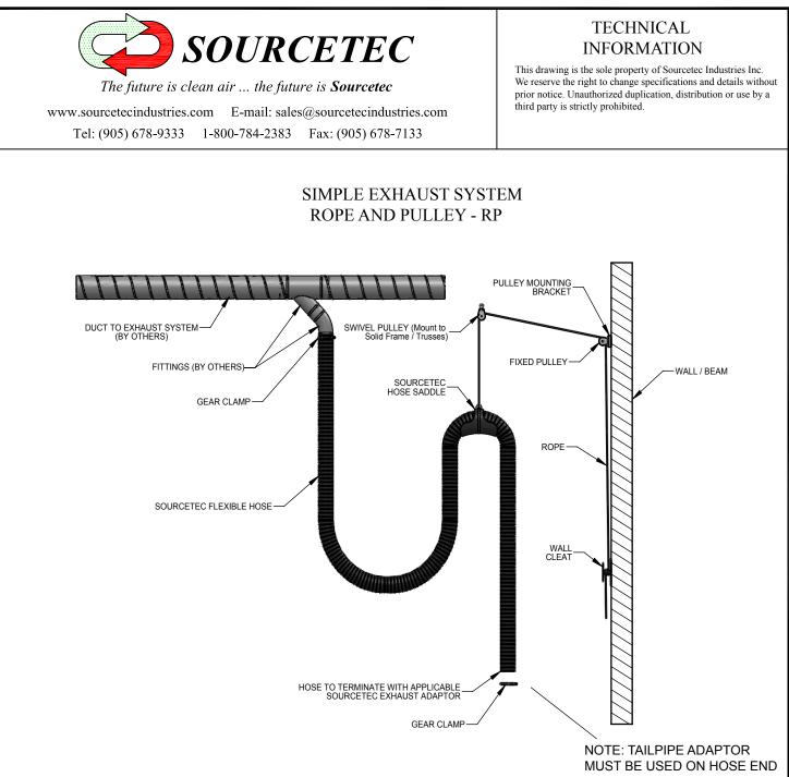
Sourcetec RP Rope and Pulley Simple Exhaust System is made up of rope and pulley mechaisms to lift and lower low temp or high temp flexible hose and hose saddle. Sourcetec RP Rope and Pulley System can be used as a single drop or hung from the main duct for a complete system. Hoses are available in 4" up to 8" Dia and lengths up to 33ft.
