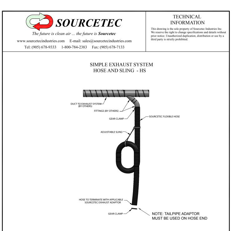
Sourcetec HS Hose and Sling Simple Exhaust System comes with no lifting mechanisms. The hose is picked up off the ground and held in place by a sling with a hook that is attached to the hose itself. Sourcetec HS Hose and Sling System can be used as a single drop or hung from the main duct for a complete system. Hoses are available in 4" up to 8" Dia and lengths up to 33ft.
