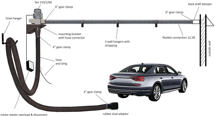
motor starter overload & disconnect \*wall mounted by others \*\*must be field wired
