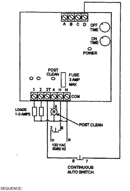
ON POWER UP, No.1 ON, THEN OFF, THEN No.2 ON THEN BACK TO No.1, AND CONTINUING FOR 9 PULSES. CLEAN LIGHT IS LIT DURING CYCLES.
