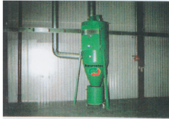
7 Various types and sizes of cyclone filters are available, with the option of manual or automatic filter cleaning.
