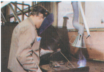
2 Flexible arms, providing both horizontal and vertical movement, can be incorporated in the system. The arms are available in various lengths.
