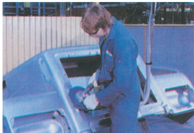
1 Central extraction for all grinding processes. The system can be adapted to suit bench grinders, belt grinders and portable angle grinders.
